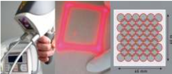
Fig. 6: An example of SOE technology: a VSP Nd:YAG laser scanner ( Fotona S-11)
